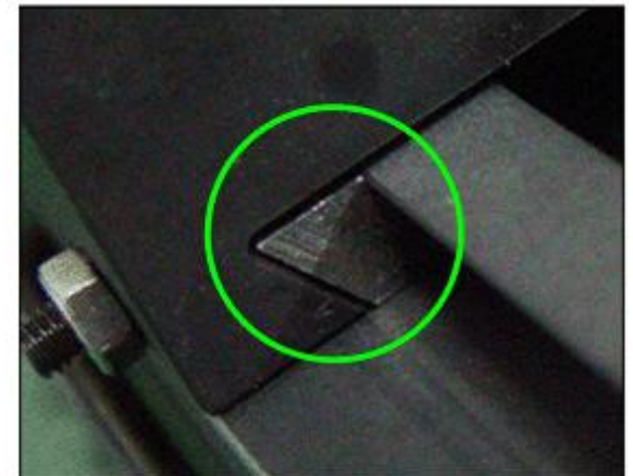
The shim for space adjustment was built in
